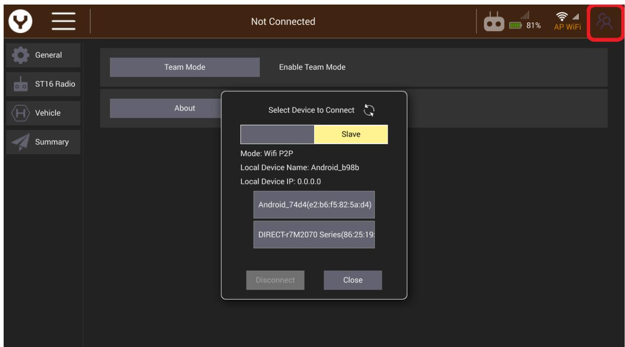
5. Select "Slave" (slave shouldn't be connected to the drone by OFDM!) and wait for Masters IP
