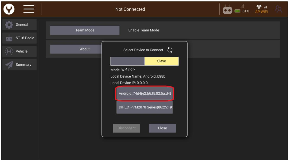
6. Accept the connection request when the window appears, you can also start the connection from Master ST16E instead of Slave
